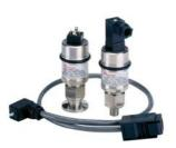
The Edwards Active Strain Gauge (ASG) is a rugged, corrosion resistant diaphragm gauge which provides accurate, gas independent measurement from 2000 mbar to 1 mbar. It can be used as a stand-alone transducer allowing OEMs and system builders to develop low cost, flexible solutions to their vacuum instrumentation needs. Alternatively, it can be connected to the TIC Instrument Controller where it can be combined with many other sensor types to provide a complete vacuum instrument solution.
