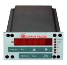
The Model 1575 Pressure Display is a low cost, microprocessor based, digital display and set-point controller for the Barocel 600, 622 and 655 capacitance manometers. The Model 1575 incorporates power supply, digital display, four user-selectable set-points, along with analog outputs in a compact 1/8 DIN package.
