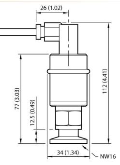
Active strain gauges are an excellent choice where accurate, gas independent, measurement of pressures around atmosphere are required, making them ideal for applications such as load locks.
